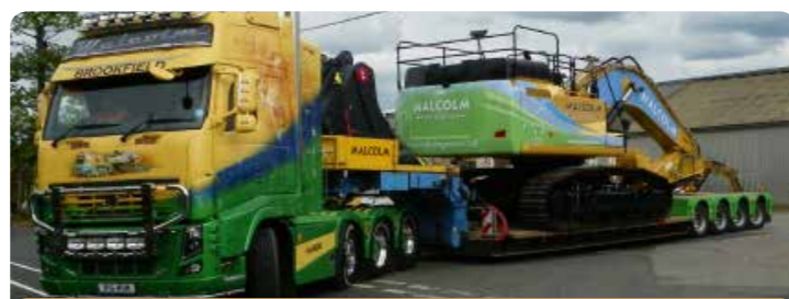
Volvo FH16 600 8x4 CAT 3 Low Loader with our CAT 349EL Tracked Excavator
